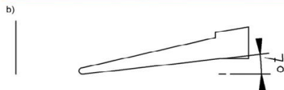
(a) Parameter for the induction coil design. (b) Induction coil with a conical angle of 7 deg.
